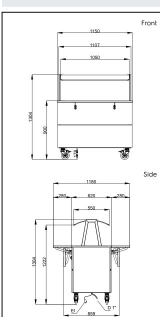
Electric Supply voltage: 322022 (F02H3AW04S) 220-240 V/1N ph/50/60 Hz Electrical power max.: 3.47 kW Water: Drain line size: 3/4" **Key Information:** N° of doors: External dimensions, Width: 1150 mm External dimensions, Depth: 1180 mm External dimensions, Height: 1304 mm Net weight: 125.5 kg Shipping height: 1334 mm Shipping width: 899 mm 1190 mm Shipping depth: Shipping volume: 1.43 m<sup>3</sup> Set temperature: +85 / +95 °C Sustainability
